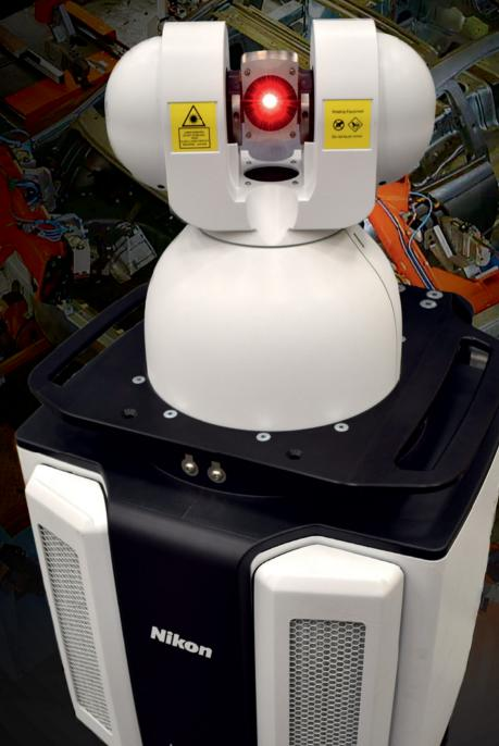
The Nikon Laser Radar is a versatile metrology system used for fast, automated and non-contact inspection of objects ranging in size from a car door to an entire aircraft wing.
