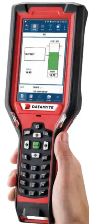
Automatically detect, display serial number, and use correct gage as characteristic's data source
