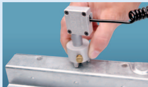
Spot Weld Indentation or Rivet Head Measurement
