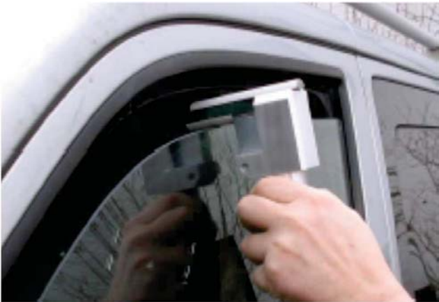
Measurement of reverse force of window panes.
